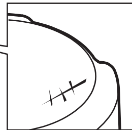
Example of Scratches on the Plated Surface
