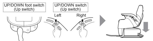
If any switch except for the legrest heater switch is pressed while the chair rotation lock is released, chair rotation is engaged and then locked.
