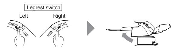
⇒ If any switch except for the legrest heater switch is pressed while the chair rotation lock is released, chair rotation is engaged and then locked.
