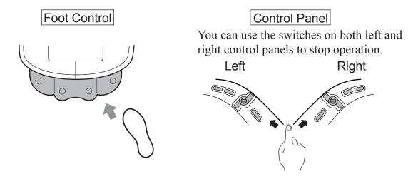
Pressing any of the switches shaded in gray will stop the operation.
