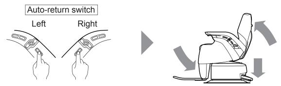
⇒ If any switch except for the legrest heater switch is pressed while the chair rotation lock is released, chair rotation is engaged and then locked.
