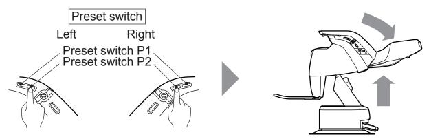
⇒ If any switch except for the legrest heater switch is pressed while the chair rotation lock is released, chair rotation is engaged and then locked.
